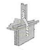
6. H6 Stud-to-Band-Joist Installation
